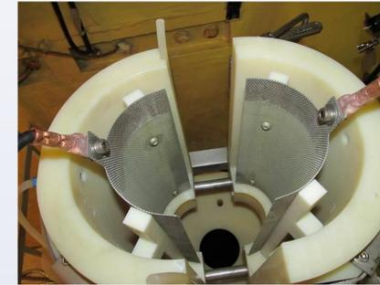
Figure 4. Electrolyser cell
