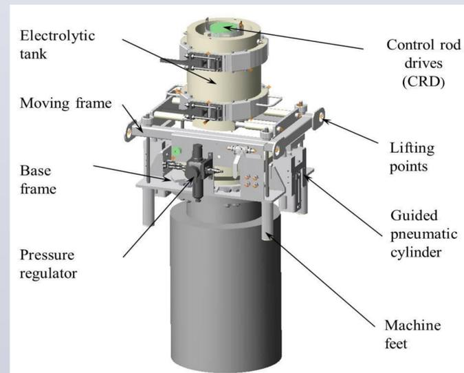
Figure 3. Schematic picture of the decontaminating equipment
