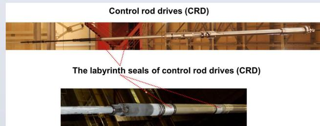
Figure 1. The control rod drives (CRD) and the labyrinth seals of CRD
