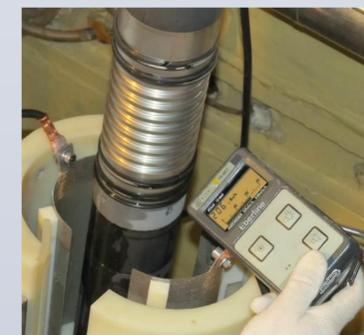
Figure 7. Dose measurement during the decontamination of the labyrinth threads
