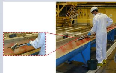
Figure 2. Manual electrochemical decontamination of CRD
