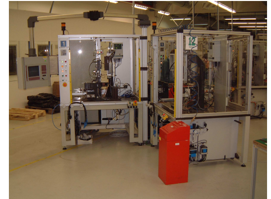
Final testing stations for quality control
